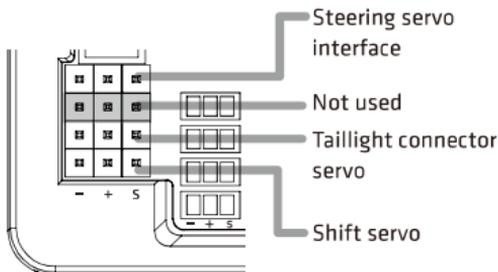
From top to bottom: Steering servo interface, not used, taillight connector servo, shift servo.
